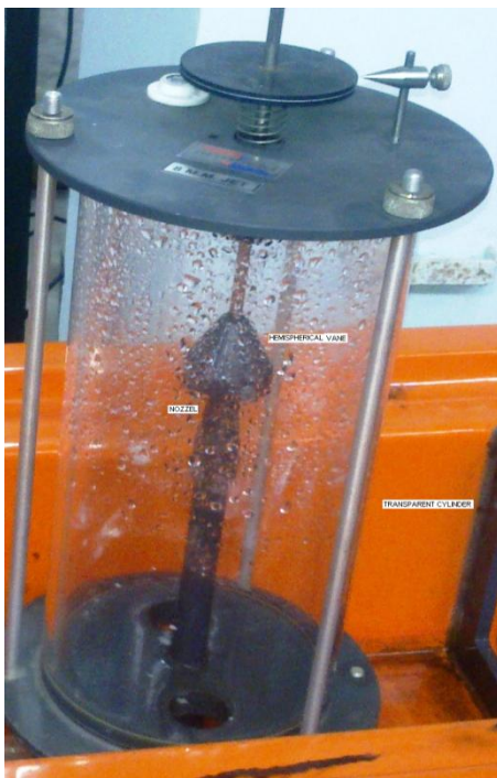
Figure 10.1 (a) Arrangement of nozzle, vane and cylinder containing power (b) Apparatus piezometer and control valve
