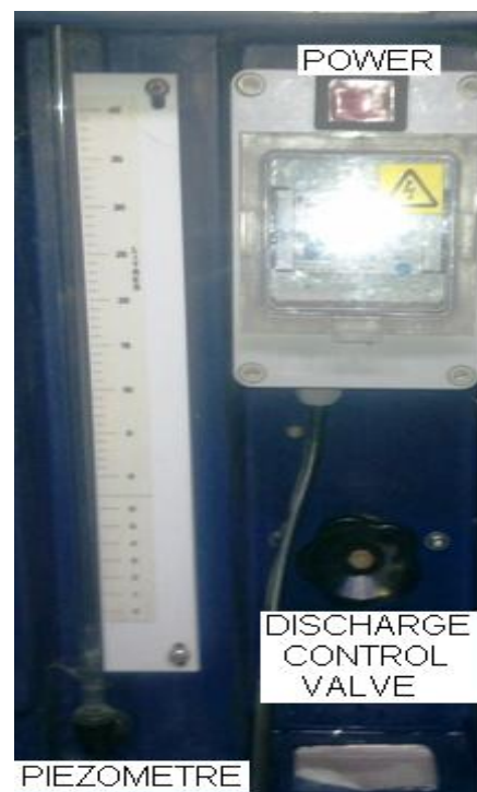
Figure 10.1 (a) Arrangement of nozzle, vane and cylinder containing power (b) Apparatus piezometer and control valve
